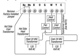
**NOTE:** Transformer Common connection not required for battery-only operation of thermostat.
