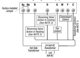
**NOTE:** 1. Transformer Common connection not required for battery-only operation of thermostat. 2. For units requiring reversing valve to be energized during heating, connect reversing valve to B terminal. 3. For units requiring reversing valve to be energized during cooling, connect reversing valve to 0 terminal.
