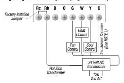
**NOTE:** 1. Transformer Common connection not required for battery-only operation of thermostat. 2. For Heating or Cooling Only System, ignore opposite connection.
